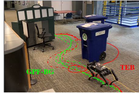
Fig. 1: Uniree A1 quadruped navigates an unknown, constrained environment. Depicts robot navigation paths for GPF-BG (green) and TEB (red).
